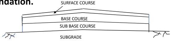
It provides adequate, smooth, durable and serviceable support for the loads imposed by traffic at all times in all weather conditions.
